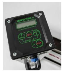
INSPECTOR-4 is portable, compact and can easily be used by a single operator. The device's intelligent built-in electronic unit calculates and displays the results immediately after the series of measurements is completed. All measured data is stored and can be downloaded to a computer via USB or Bluetooth connection. The results can also be read to the user's mobile phone and forwarded via e-mail to off-site staff for real-time verification against expected results.
