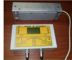
The device comes with two separate units – slope sensor with signal precision amplifier and slope measuring and control unit – that are connected by a flexible cable. The slope sensor unit is connected to the bulldozer bucket and the slope measuring and control unit is attached to the window of the cabin, allowing the operator to view the measurement results and alarms directly from the cabin.
