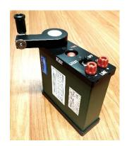
The integrated line tester verifies the line's integrity and uses a two color LED that indicates to the user whether the resistance of the line and detonators is below 450  $\Omega$ . For safety reasons, the line tester current is limited to 1mA.
