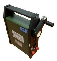
The integrated line tester verifies the line's integrity and uses a two color LED that indicates to the user whether the resistance of the line and detonators is below or above 700  $\Omega$ , in accordance with Class 1 detonators. For safety reasons, the line tester current is limited to 1mA.
