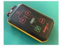
tester current is limited to 1mA. Three digit LED display helps to safely control the blasting line of the electric detonators.
