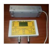
The device comes with two separate units – slope sensor with signal precision amplifier and slope measuring and control unit – that are connected by a flexible cable. The slope sensor unit is connected to the grader blade and the slope measuring and control unit is attached to the window of the cabin, allowing the operator to view the measurement results and alarms directly from the cabin.
